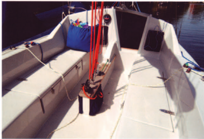
A large cockpit provides plenty of crew space and also simplifies sail handling by allowing easy access to the foot of the mast
