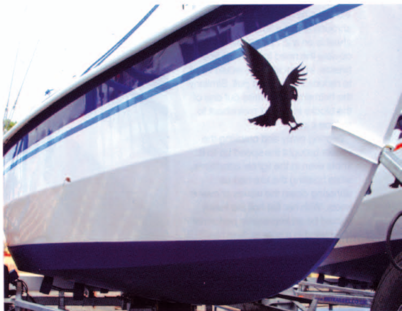
Sharp chines: the flat sections contribute to high form stability
