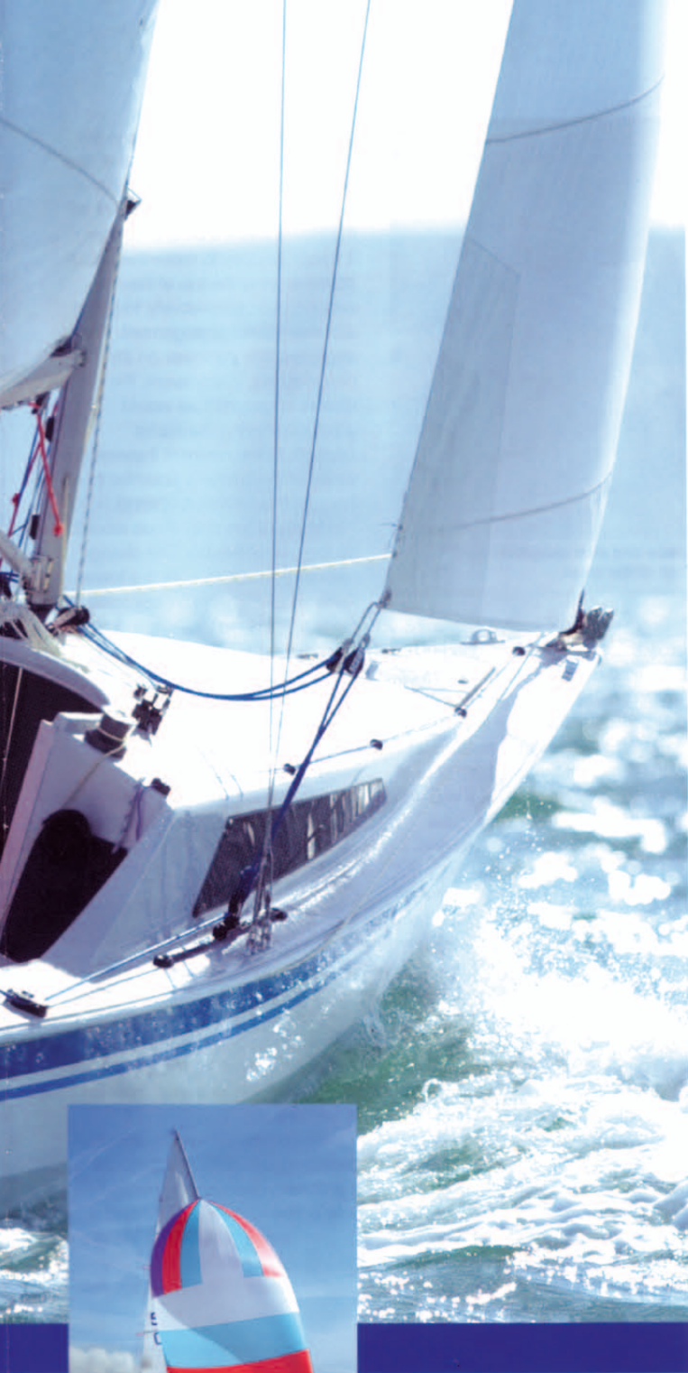
Sharp chines: the flat sections contribute to high form stability
