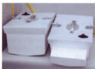
Fairing plugs fit into the bottom of the hull to eliminate turbulence when the outboard is raised
